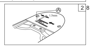
To adjust the position of feed dog, move feed dog to the front end of throat plate, Loosen Screw A (See Fig 29b), move feed dog support B in the direction shown by arrow (Fig.29a) to adjust. After adjustment tighten Screw(A).
