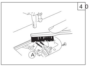
2. Cleaning the rotating Clean off all the dust around the rotating hook (A), and clean the bobbin case with soft cloth.
