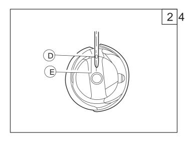
2. Adjusting rotating hook point timing with needle.
