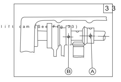
3. Installing feed cam Continously turn balance wheel, take Screw (B) as for standard, the center of Screw (C) is slightly a little higher than the center of Screw (B).
