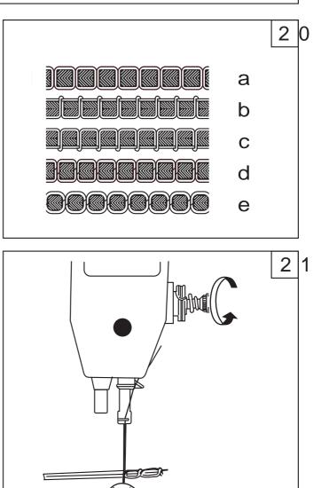
(B) The needle thread tension is too weak or the bobbin thread is too strong, turn the tension regulating thumb nut clockwise to make the needle thread get more tension or turn the bobbin case tension regulating screw counter clockwise with small plastic screw driver to make the bobbin thread get less tension (Fig.22)
